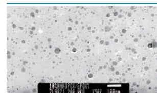
■ ARE-310 Nano-silica is uniformly dispersed in epoxy resin. SEM photo by Dr. J.H. Koo, University of Texas at Austin
