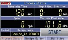
Displays real-time revolution speed and vacuum pressure
